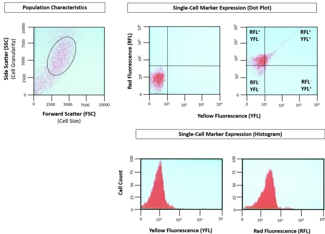
**Figure 6:** Typical flow cytometry plots for assessing single cells and cell population characteristics. Forward and side scatter are used to gate a population of interest based on size and granularity respectively. The gated population can then be assessed by co-expression or single expression of markers of interest using a fluorescence/antibody-based system. The total number of cells and their expression profile can then be quantified.
