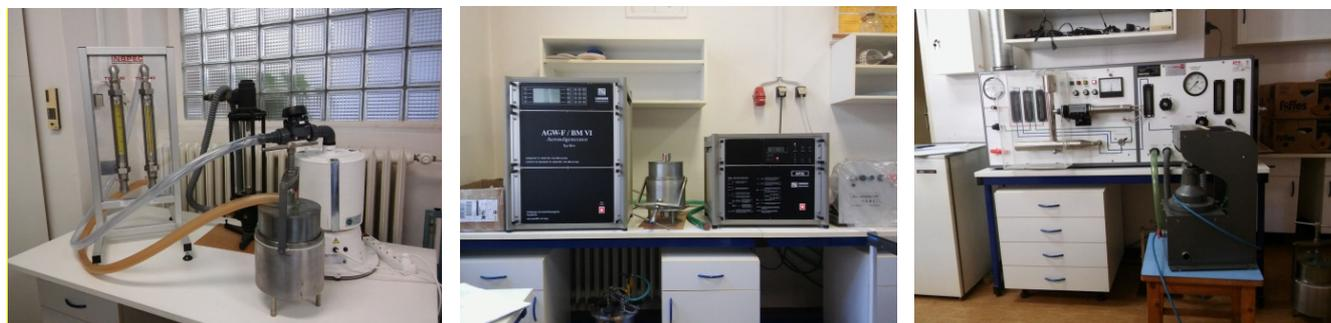
Figure 19: Measurement device for respiratory resistance and aerosol penetration for NaCl and paraffin oil (b) Sodium chloride test - Breakthrough of NaCl after 3 minutes. Flow rate 45 l/min.
