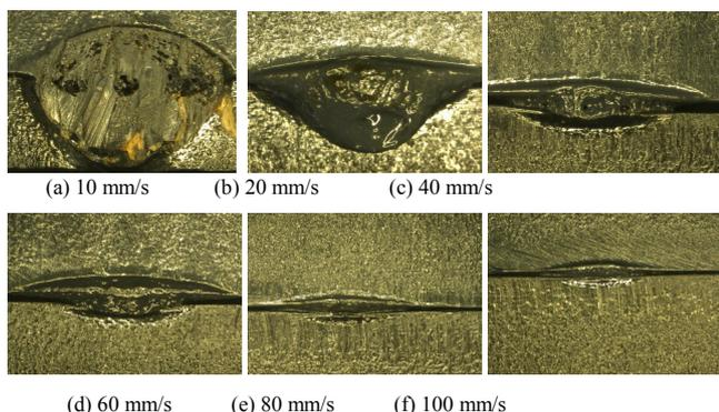
**Figure 13:** Molten depths in the transparent and absorbing PC obtained in welding experiment; magnification of 50X.
