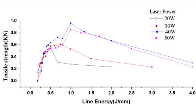
**Figure 14:** Transparent part thickness 1 mm, weld strength as a function of line energy.
