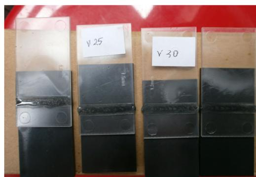
Figure 5: Welding 20~30 mm/s, laser power 40 W, slight degradation of the weld joint occur.
