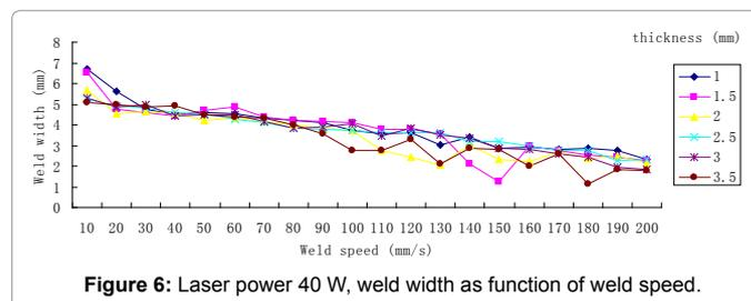
Figure 6: Laser power 40 W, weld width as function of weld speed.
