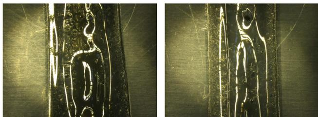
**Figure 12:** Laser power 50W, welding speed 40 mm/s; (a) transparent part thickness 1 mm; (b) transparent part thickness 1.5 mm.
