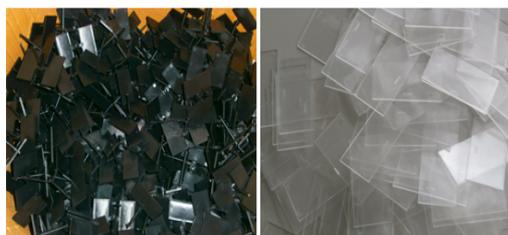
Figure 2: Injection molded of transparent and absorbent parts.
