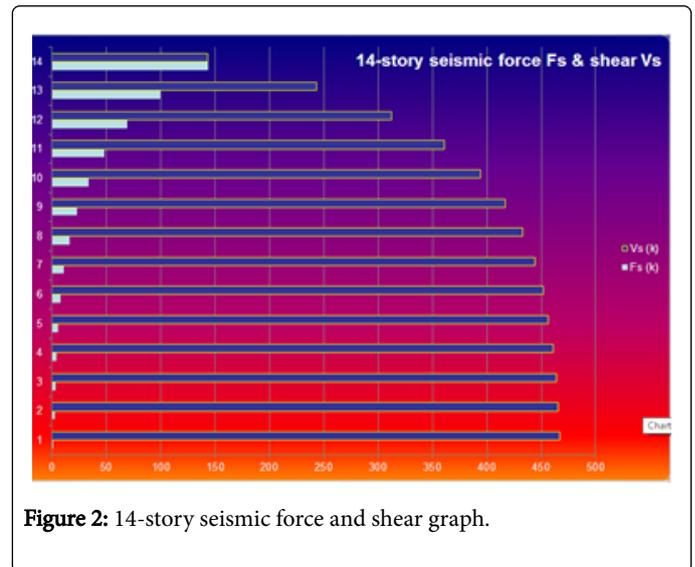
Figure 2: 14-story seismic force and shear graph.
