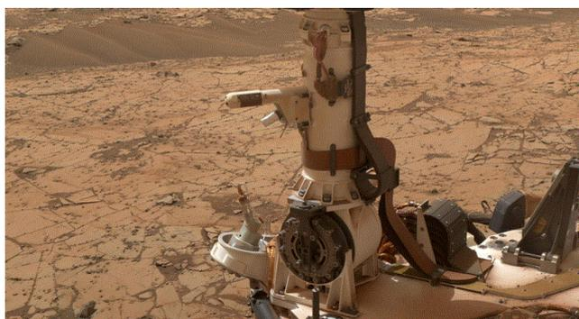
Figure 1: Image of REMS's boom 2 on Curiosity's Mast.
