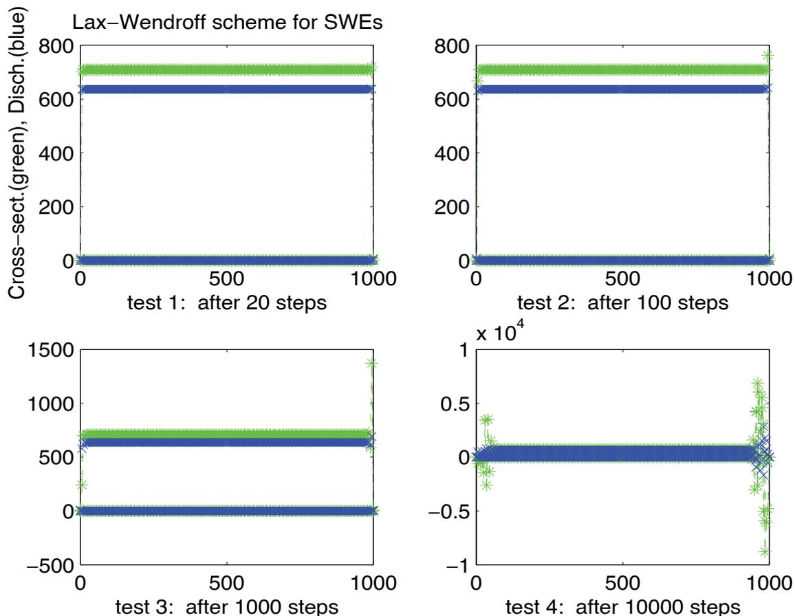
**Figure 1:** Cross-section (in green) and Discharge (in blue) profiles obtained from the Lax-Wendroff scheme for 1D complete shallow water flow in a prismatic channel.
