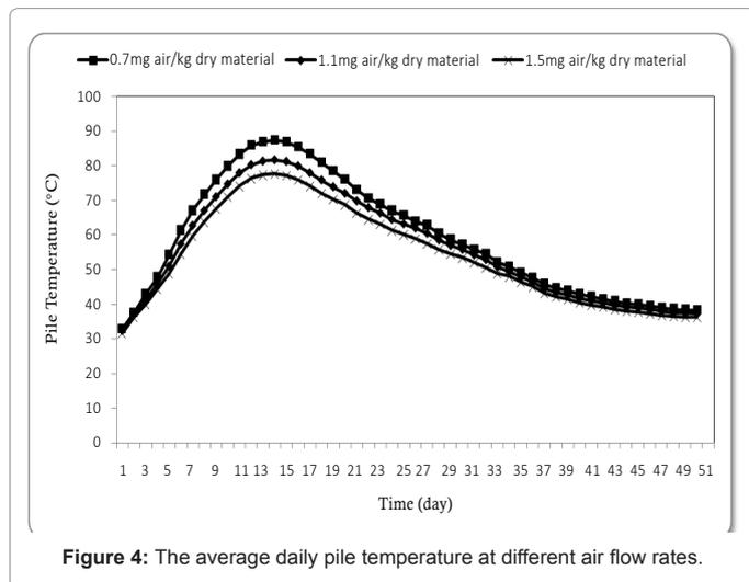
Figure 4: The average daily pile temperature at different air flow rates.
