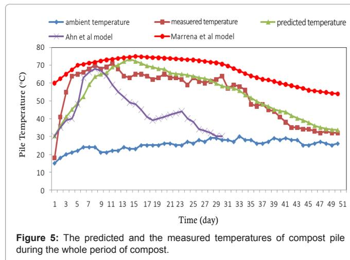
Figure 5: The predicted and the measured temperatures of compost pile during the whole period of compost.
