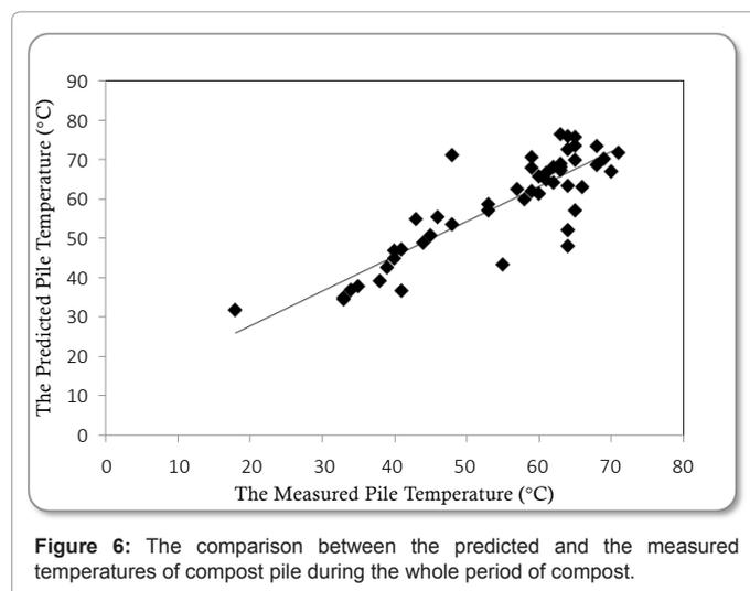
Figure 6: The comparison between the predicted and the measured temperatures of compost pile during the whole period of compost.
