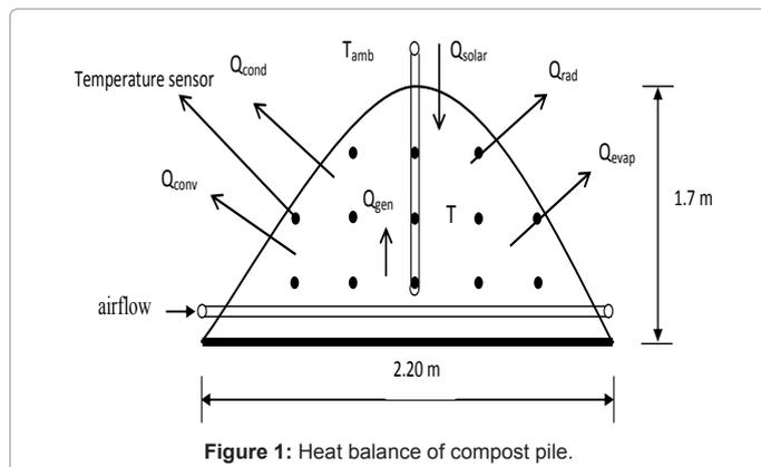
Figure 1: Heat balance of compost pile.
