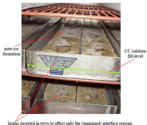
Figure 3: Freezing-thawing.
