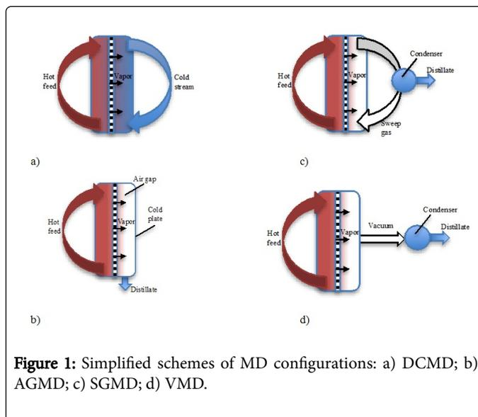
**Figure 1:** Simplified schemes of MD configurations: a) DCMD; b) AGMD; c) SGMD; d) VMD.
