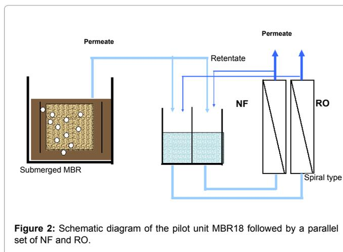
Figure 2: Schematic diagram of the pilot unit MBR18 followed by a parallel set of NF and RO.
