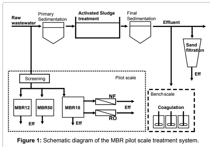
Figure 1: Schematic diagram of the MBR pilot scale treatment system.
