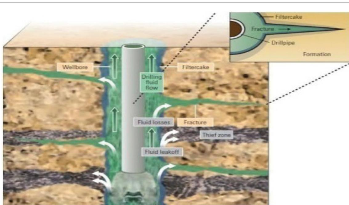
Figure 1: Schematic illustration of formation of cracks during petroleum drilling operations.
