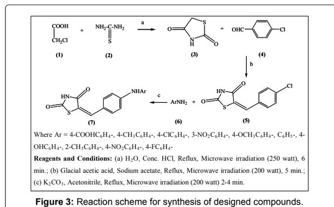
Figure 3: Reaction scheme for synthesis of designed compounds.
