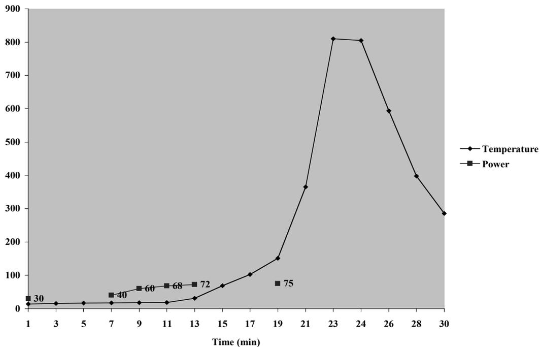
**Figure 1:** Time-temperature-power profile that was found to be ideal to obtain best mechanical and microstructural properties in the sintered dental crowns. The horizontal axis indicates time in minutes and the vertical axis the temperature in °C.
