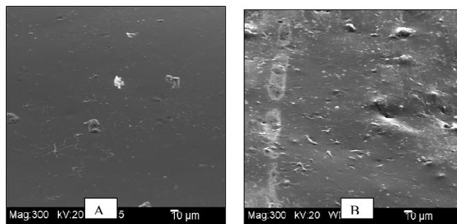
**Figure 3:** The figure A depicts the glassy microstructure of samples sintered according to the ideal thermal profile and when faster sintering were attempted in both conventional and microwave furnace there was a distinctively poor glass phase with improper crystal precipitation.
