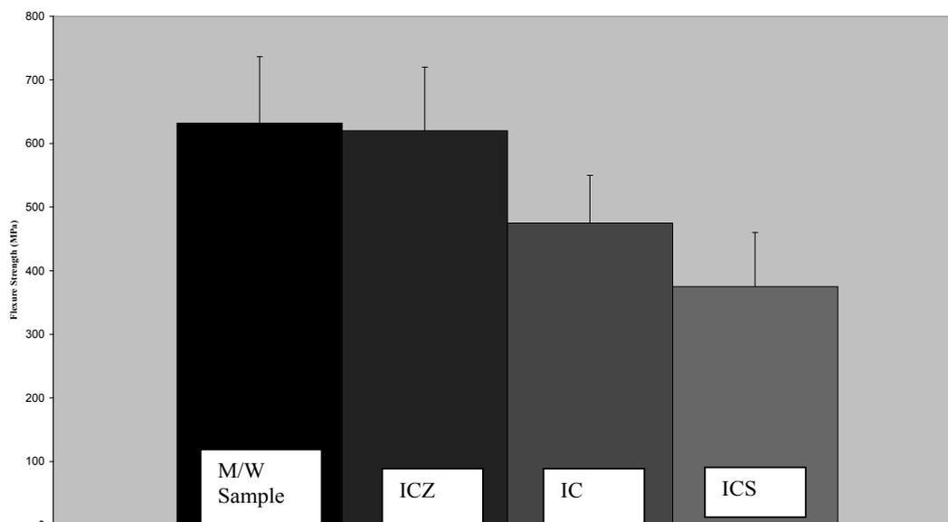
**Figure 4:** The modulus of Rupture for the M/W sintered samples were  $632 \pm 105$ MPa and were compared against the published values of Inceram Zirconia (ICZ), Inceram Alumina (IC) and Inceram Magnesium Aluminum Spinel (ICS).
