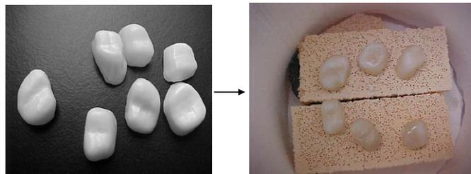
**Figure 2:** Using the ideal sintering profile the presintered copings (left) were sintered and restorations with optimum esthetics and completed sintering were obtained (right).
