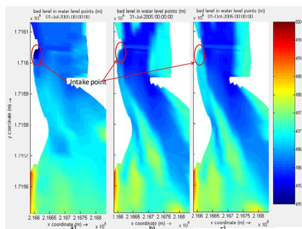
**Figure 9:** River morphology change at Fota diversion intake: (a) at the beginning, (b) after 1 month and (c) after one year simulation.
