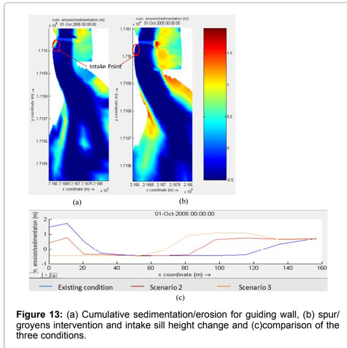
**Figure 13:** (a) Cumulative sedimentation/erosion for guiding wall, (b) spur/groynes intervention and intake sill height change and (c) comparison of the three conditions.
