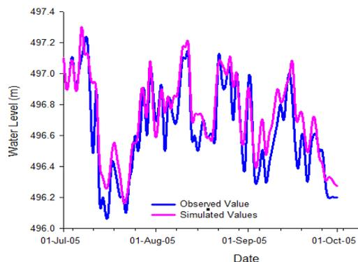
**Figure 7:** Daily water level for observed and simulated at Fota gauge station (2005).
