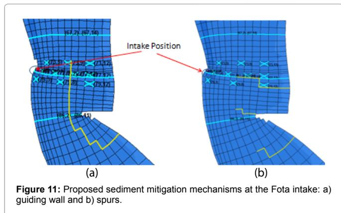
Figure 11: Proposed sediment mitigation mechanisms at the Fota intake: a) guiding wall and b) spurs.
