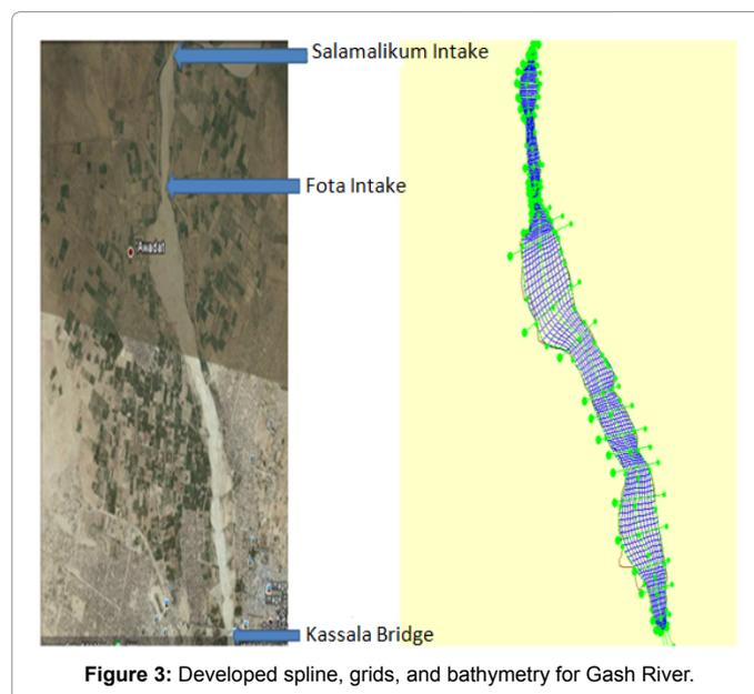
numerical grid and bathymetry of the river were established. The grid orthogonalized and smoothed to reach representative schematization of the flow pattern in the study area. The generated grids for the river have the following properties:
