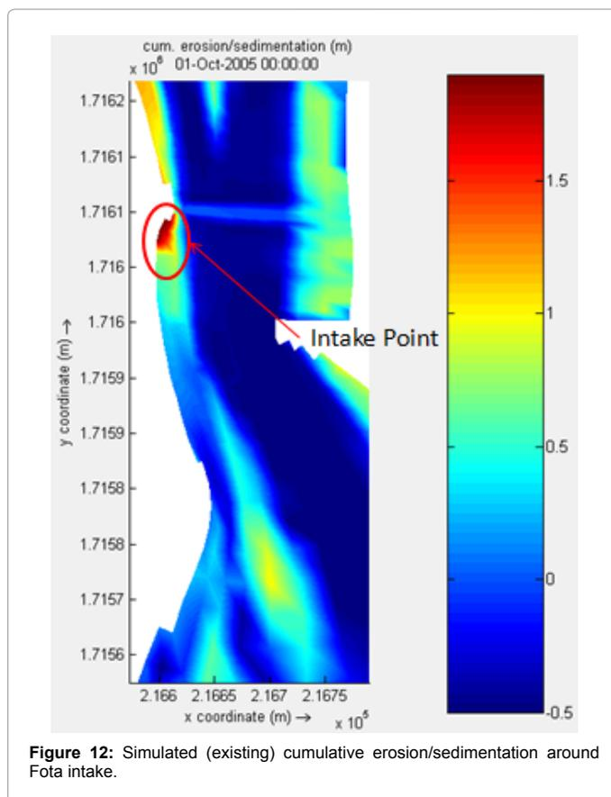
Figure 12: Simulated (existing) cumulative erosion/sedimentation around Fota intake.
