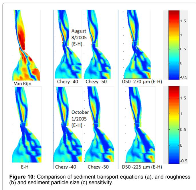
Figure 10: Comparison of sediment transport equations (a), and roughness (b) and sediment particle size (c) sensitivity.
