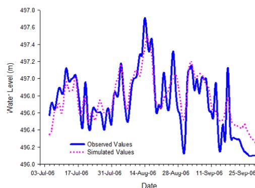
**Figure 8:** Daily water level for observed and simulated at Fota gauge station (2006).
