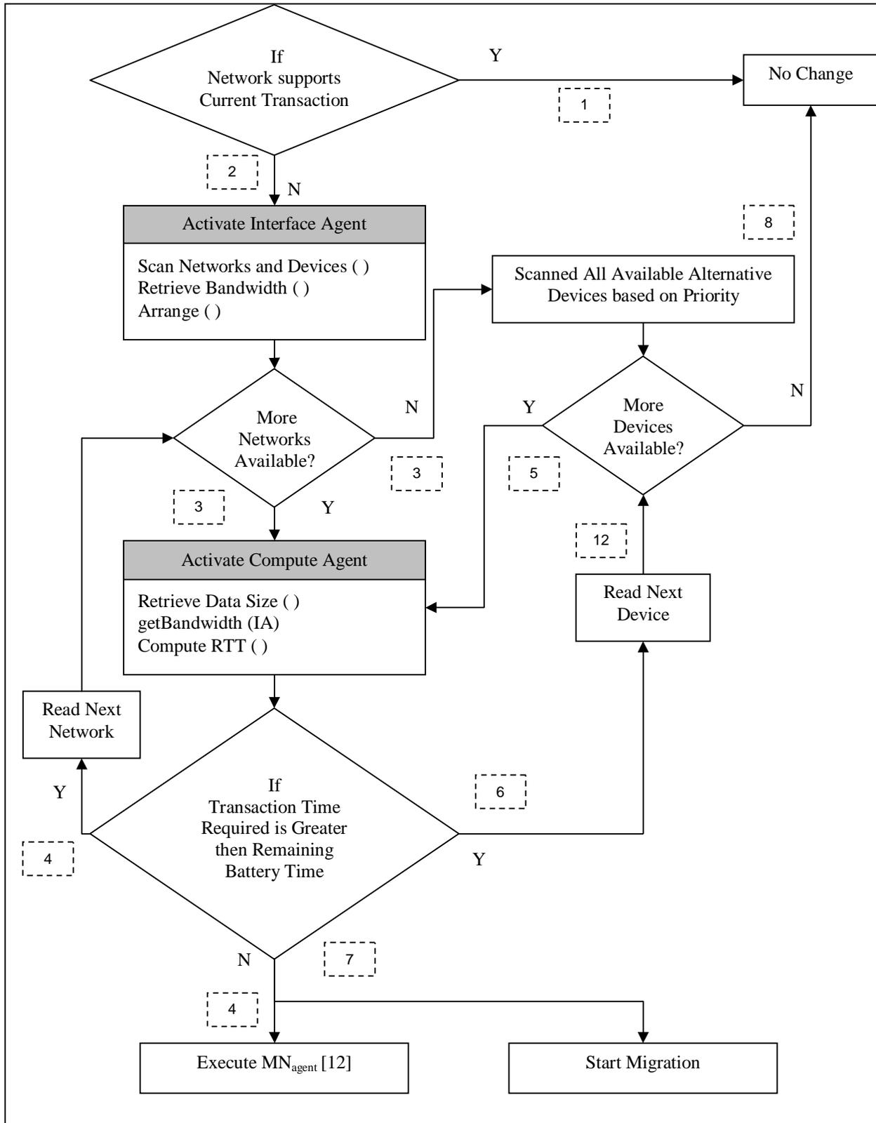
Figure 3: State Diagram of MAEF: The Proposed Work
