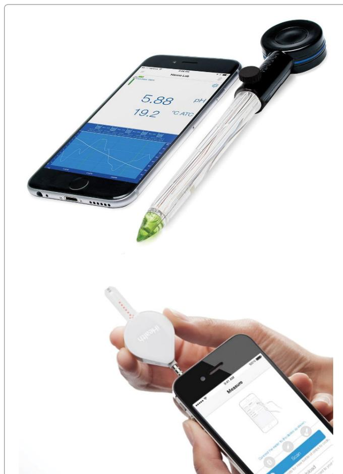
**Figure 1:** The examples of commercially available mobile-phone-based portable analytical devices: A - The pH probe with Bluetooth technology (<http://hannainst.com/halo>), B - The electrochemical portable glucose meter employing blood glucose test stripe, which plugs directly into the smartphone's headphone jack, and displays results directly on the phone screen [11].
