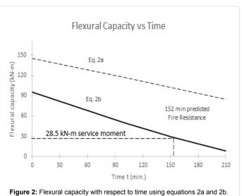
within 20% of the actual failure time of 128 minutes obtained through experimentation.
