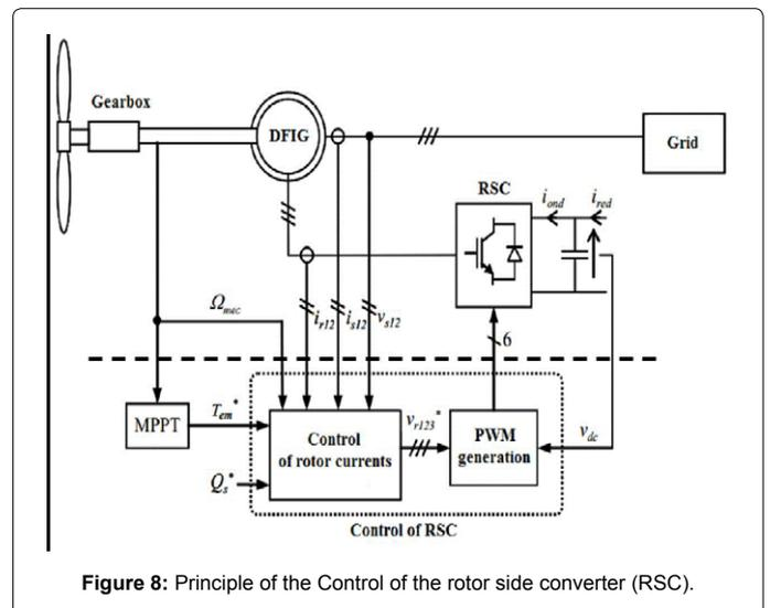
Figure 8: Principle of the Control of the rotor side converter (RSC).
