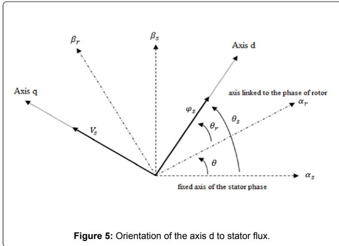
Figure 5: Orientation of the axis d to stator flux.
