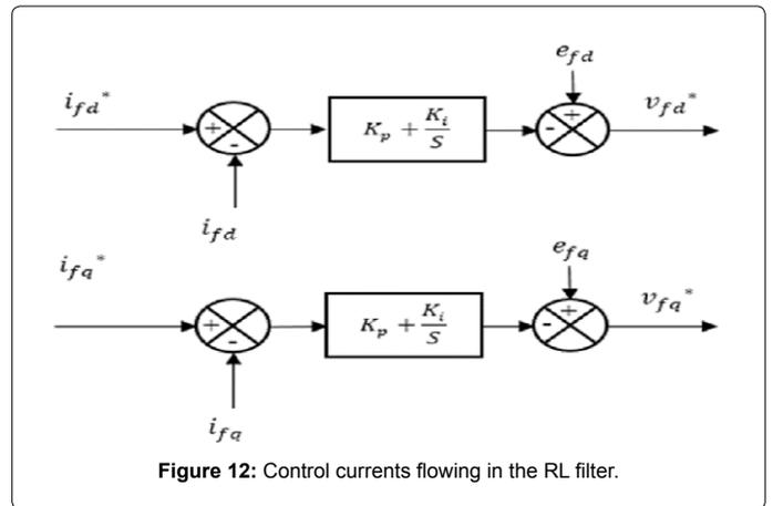
Figure 12: Control currents flowing in the RL filter.
