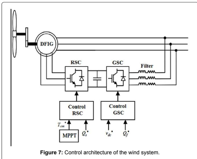
Figure 7: Control architecture of the wind system.
