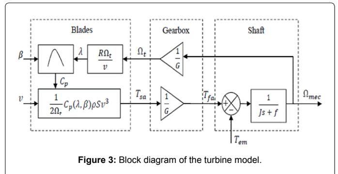
Figure 3: Block diagram of the turbine model.
