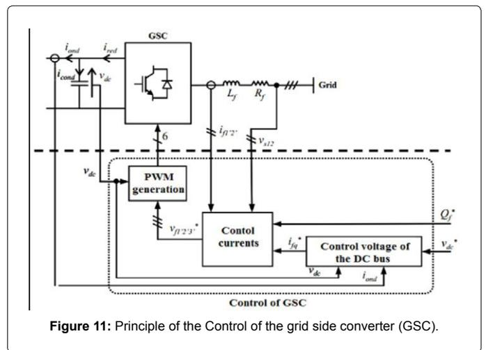
Figure 11: Principle of the Control of the grid side converter (GSC).
