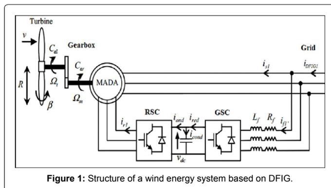
Figure 1: Structure of a wind energy system based on DFIG.
