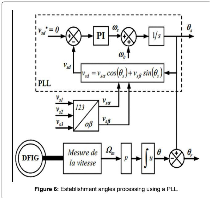
Figure 6: Establishment angles processing using a PLL.
