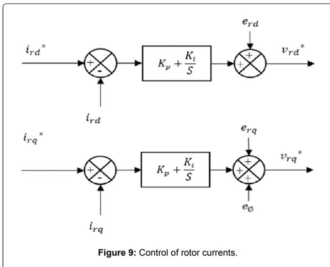
Figure 9: Control of rotor currents.
