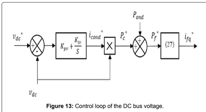
Figure 13: Control loop of the DC bus voltage.
