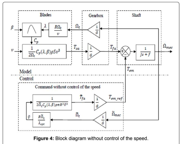
Figure 4: Block diagram without control of the speed.
