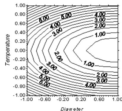
Figure 5: Effect of notch diameter and temperature on the elongation.
