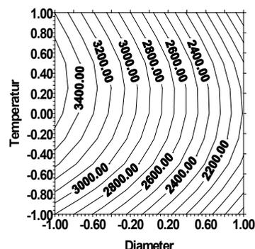
Figure 4: Effect of notch diameter and temperature on the tensile fracture load.
