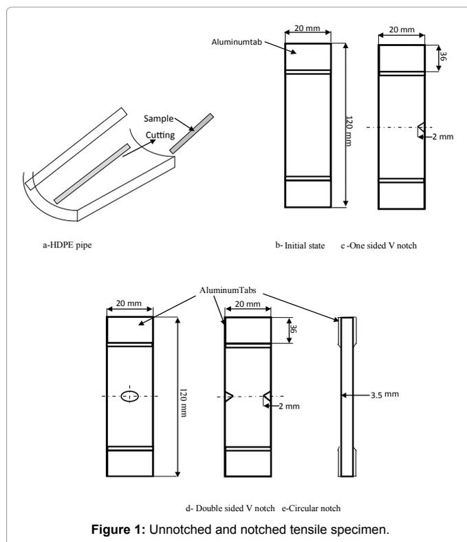
Figure 1: Unnotched and notched tensile specimen.
