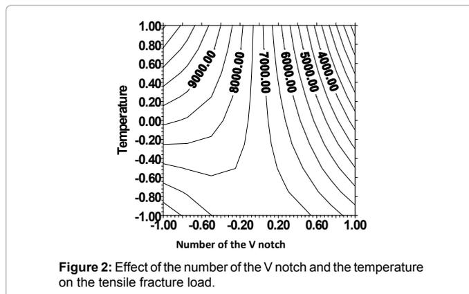
Figure 2: Effect of the number of the V notch and the temperature on the tensile fracture load.
