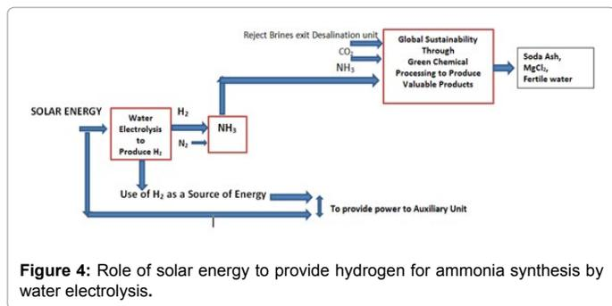
Figure 4: Role of solar energy to provide hydrogen for ammonia synthesis by water electrolysis.
