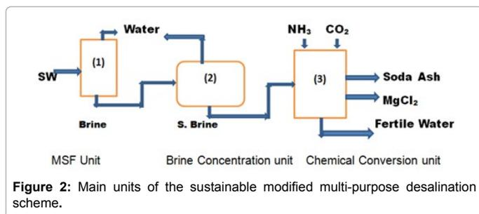
Figure 2: Main units of the sustainable modified multi-purpose desalination scheme.
