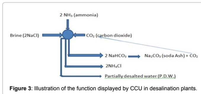
Figure 3: Illustration of the function displayed by CCU in desalination plants.
