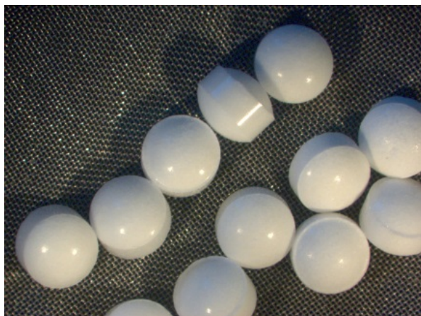
Figure 1: Spherical mini-tablets for pediatric use (3.6 mm diameter).
