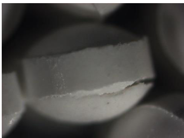
Figure 2: Delaminating on spherical mini-tablets.
