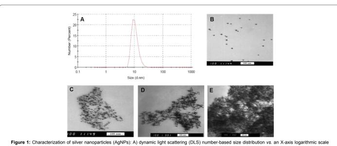
Figure 1: Characterization of silver nanoparticles (AgNPs): A) dynamic light scattering (DLS) number-based size distribution vs. an X-axis logarithmic scale (diameter in nm; d.nm); B) transmission electron micrographs (TEM) image of the AgNP stock suspension; and also TEM images of AgNPs in the bacterial culture media at C) 25, D) 100 & E) 200 mg/L concentrations.
