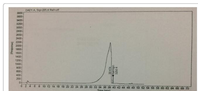
**Figure 1:** HPLC chromatogram obtained from the dimethyl sulfoxide (DMSO) fraction of grapefruit rind. The main peak is that of naringin, which is the dominant phenolic compound in grapefruit, RT=39.47.
