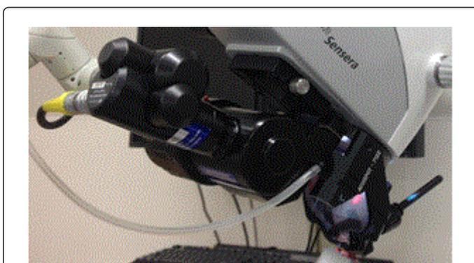
**Figure 3:** A micromanipulator which couples the CO<sub>2</sub> laser and the operating microscope. Note the joystick on the right-hand side, which controls the aiming beam of the laser
