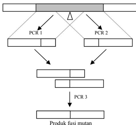
**Fig. 6.** Site-directed mutagenesis by SOE which involves PCR-amplification of a wild-type gene using two overlapping mutagenic primers. The PCR products of PCR reaction 1 and 2 are overlapping fragments, which are joined together in the third PCR reaction, thereby generating mutated variants of wild-type protein. Copied from van der Oost and de Graaff, 2002.
