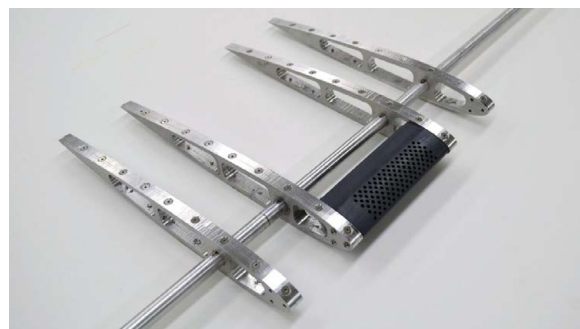
Figure 2: Assembly of NACA 0012 model with aluminum sheet metal and latex skin removed; the dynamic roughness actuation section is located in the leading edge region of the two center ribs. The shaft through the quarter chord location acts as the rotation axis.
