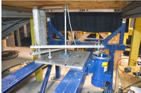
Figure 3: Airfoil oscillation mechanism mounted below the wind tunnel test section showing both the four bar linkage as well as the DC motor.
