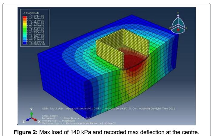
Figure 2: Max load of 140 kPa and recorded max deflection at the centre.
