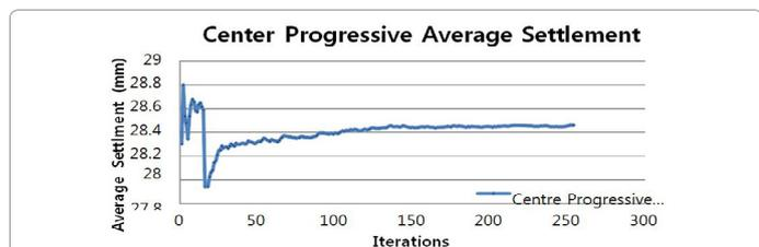
Figure 5: Internal angle of friction varied, centre progressive average settlement.
