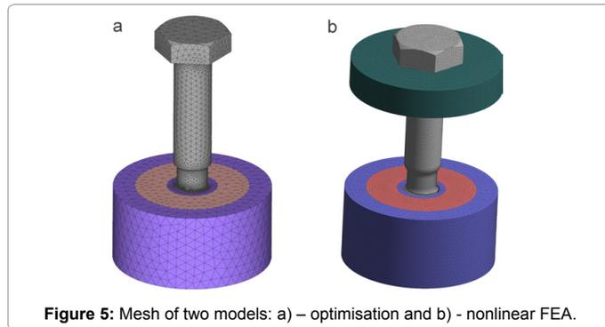
Figure 5: Mesh of two models: a) – optimisation and b) - nonlinear FEA.
