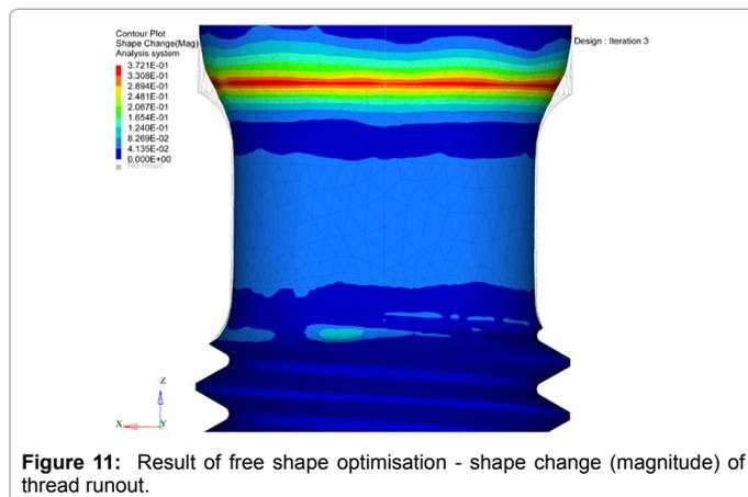
Figure 11: Result of free shape optimisation - shape change (magnitude) of thread runout.
