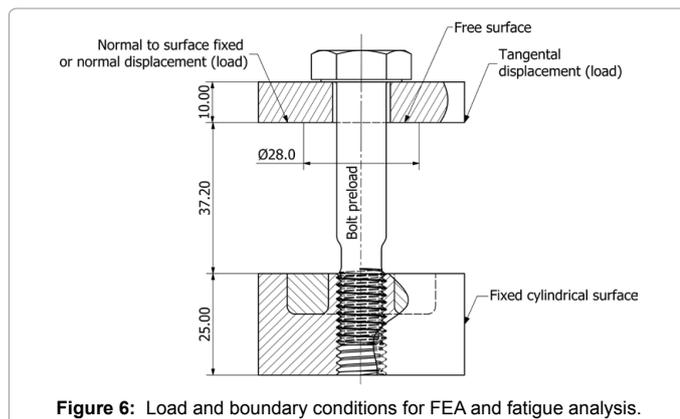
Figure 6: Load and boundary conditions for FEA and fatigue analysis.
