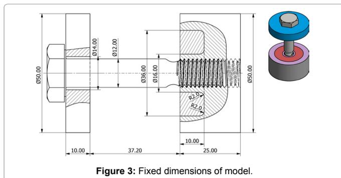
Figure 3: Fixed dimensions of model.
