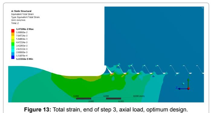
Figure 13: Total strain, end of step 3, axial load, optimum design.
