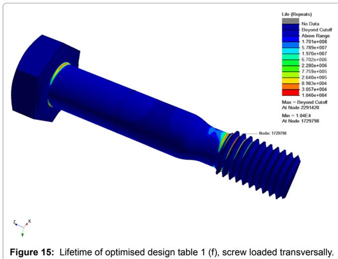
Figure 15: Lifetime of optimised design table 1 (f), screw loaded transversally.
