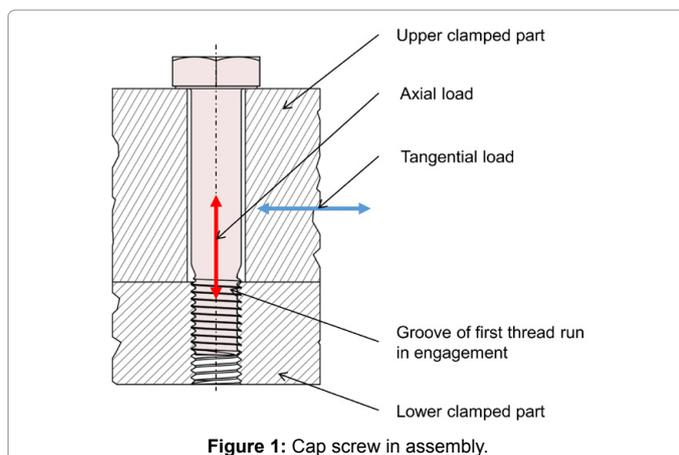
Figure 1: Cap screw in assembly.
