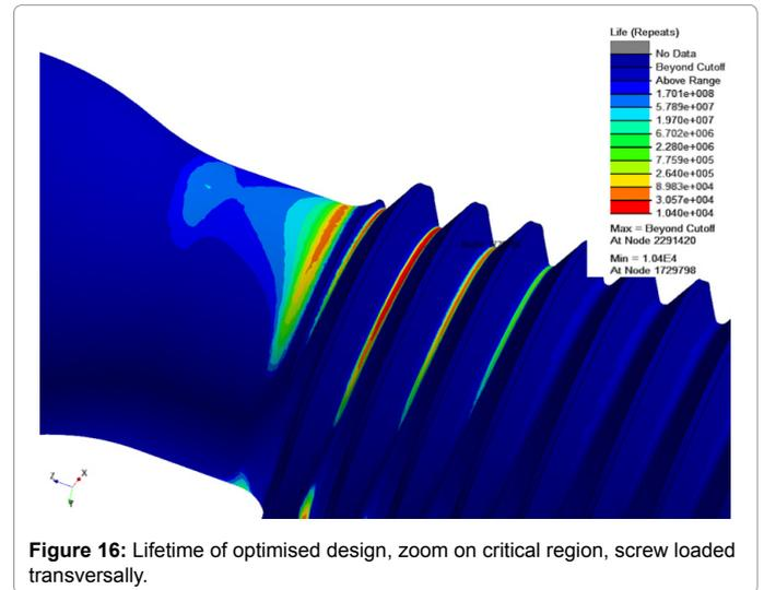
Figure 16: Lifetime of optimised design, zoom on critical region, screw loaded transversally.
