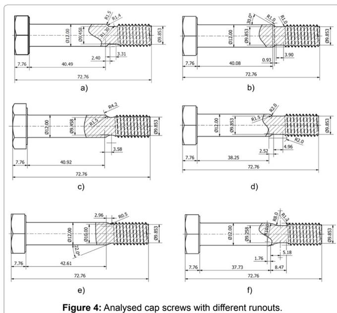
Figure 4: Analysed cap screws with different runouts.
