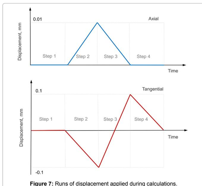
Figure 7: Runs of displacement applied during calculations.
