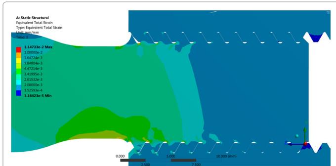
Figure 14: Total strain, end of step 3, tangential load, optimum design.
