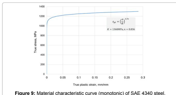
Figure 9: Material characteristic curve (monotonic) of SAE 4340 steel.
