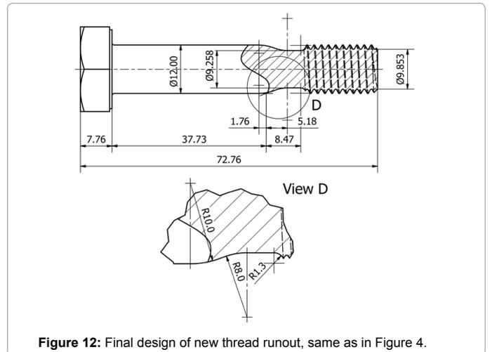
Figure 12: Final design of new thread runout, same as in Figure 4.
