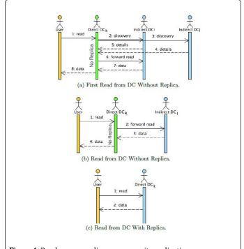
Figure 4: Read sequence diagrams on write replication.
