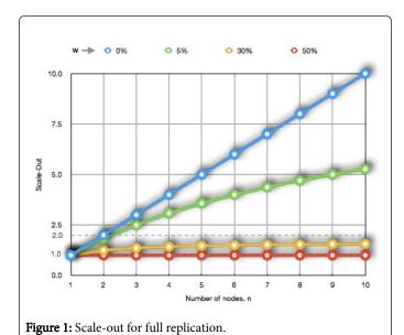
If n=1, with no replication, then all capacity is used in local work and any increase in the number of nodes correlates to a linear increase in total local work capacity, which it is also corroborated by the scaleout, blue line on Figure 1. But it also corresponds to losing the recovery capability provided with replication, which may reduce availability, and increase access times.
