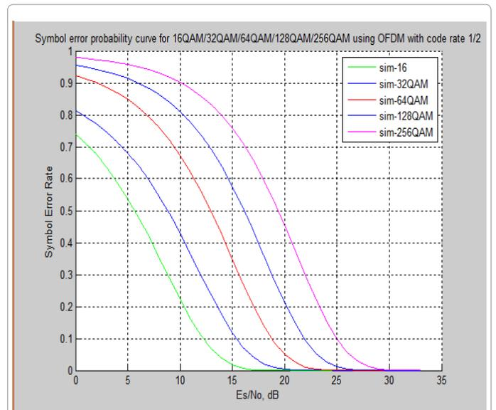
Figure 3: SER comparison of different QAM with code rate 1/2 code.
