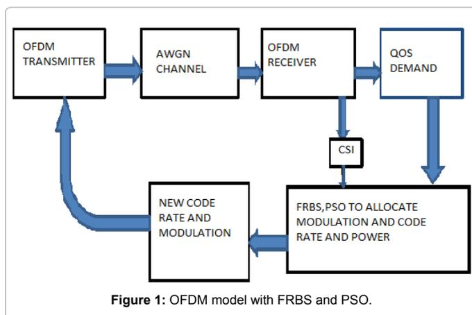
Figure 1: OFDM model with FRBS and PSO.
