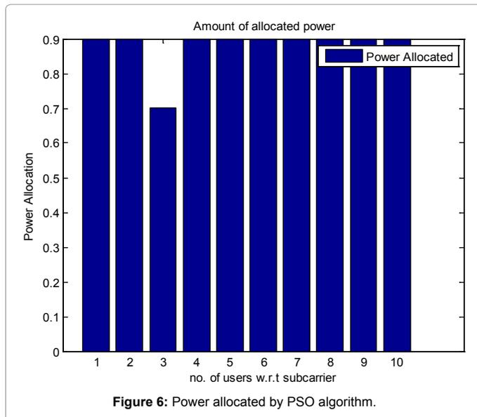
optimization of code rate and modulation. Higher numbered CMP reflects a higher throughput. PSO is used for allocation of power for each sub-channel depending upon the channel condition. After using FRBS in OFDM system it will give optimal modulation and Code rate. Thus y using FRBS and PSO optimal power allocation can be done with specified modulation techniques for specified sub channel.
