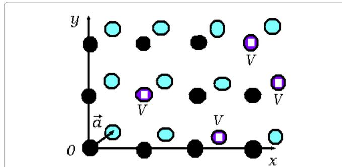
**Figure 1:** Schematic of a non-ideal two-dimensional two-sublattice system of microcavities for the case of a square Bravais lattice, “V” denotes vacancies.
