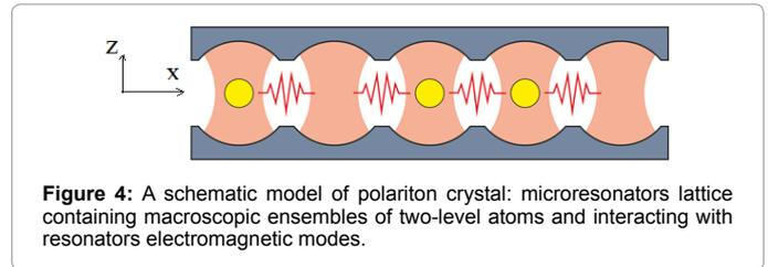
Figure 4: A schematic model of polariton crystal: microresonators lattice containing macroscopic ensembles of two-level atoms and interacting with resonators electromagnetic modes.
