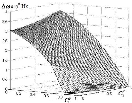
Figure 3: Vacancies concentration dependence of the photonic gap width  $\Delta\omega(C_1^v, C_2^v)$  in the studied microcavity supersystem.
