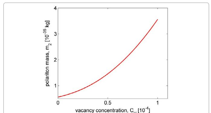
Figure 5: The dependence of polaritonic mass  $m_2$  on vacancies  $C_v$  in the imperfect superlattice of coupled microresonators.
