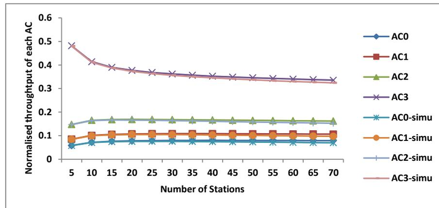
Fig 4: Comparison of Analytical Throughput Value with Simulation Result for RTS-CTS Mode.
