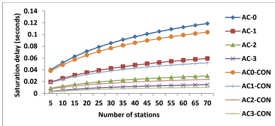
Fig 7: RTS/CTS delay of standard EDCA (AC-0, AC-1, AC-2, and AC-3) and EDCA with frame-concatenation and block-acknowledgement (AC0-CON, AC1-CON, AC2-CON, AC3-CON)
