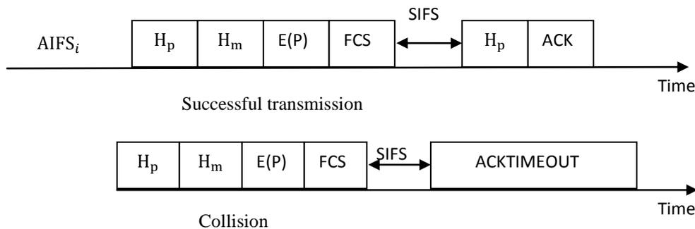
Fig 3(b): Timing Sequence for Transmission of Basic Mode of Standard EDCA for  $i_{th}$  AC.
