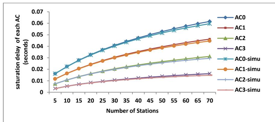
Fig 5: Comparison of Analytical Delay Value with Simulation Result for RTS-CTS Mode.
