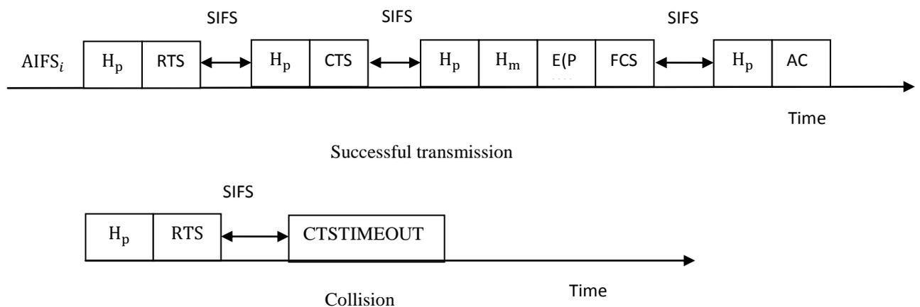
Fig 3(a): Timing Sequence for Transmission of RTS/CTS Mode of Standard EDCA for  $i_{th}$  AC.
