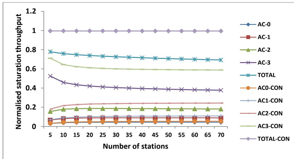
Fig 6: RTS/CTS throughput of standard EDCA (AC-0, AC-1, AC-2, AC-3, TOTAL) and EDCA with frame-concatenation and block-acknowledgement (AC0-CON, AC1-CON, AC2-CON, AC3-CON, TOTAL-CON).
