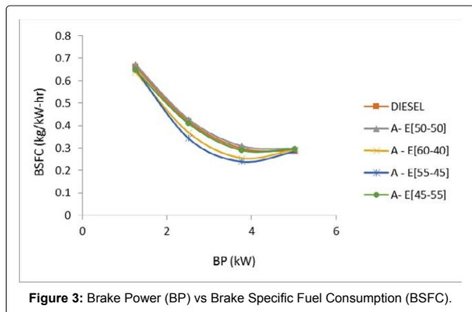
Figure 3: Brake Power (BP) vs Brake Specific Fuel Consumption (BSFC).
