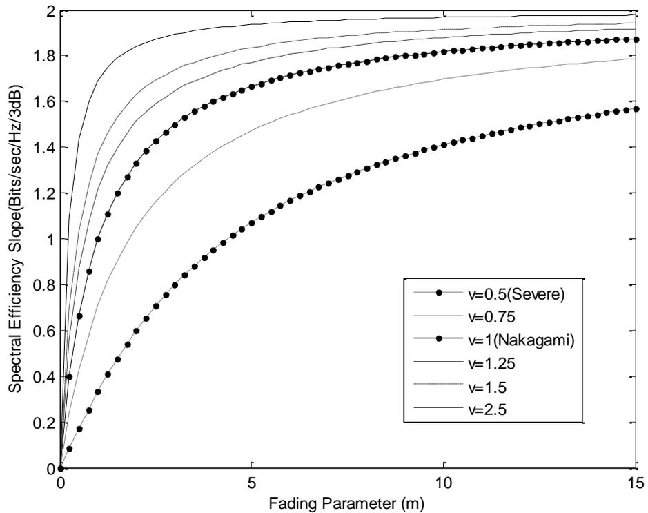
Fig. 2: Spectral Efficiency Curve Slope in Different Generalized Fading Conditions
