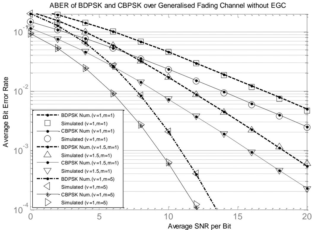
**Fig. 3:** ABER vs Average SNR of BDPSK and CBPSK Without Diversity Combining
