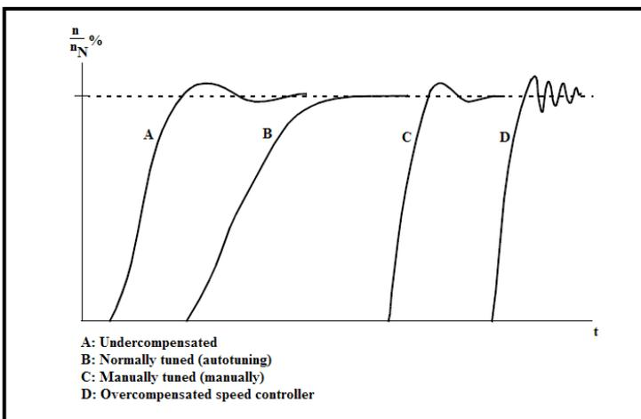
**Figure 3: Speed Responses at a Speed Reference Step**
