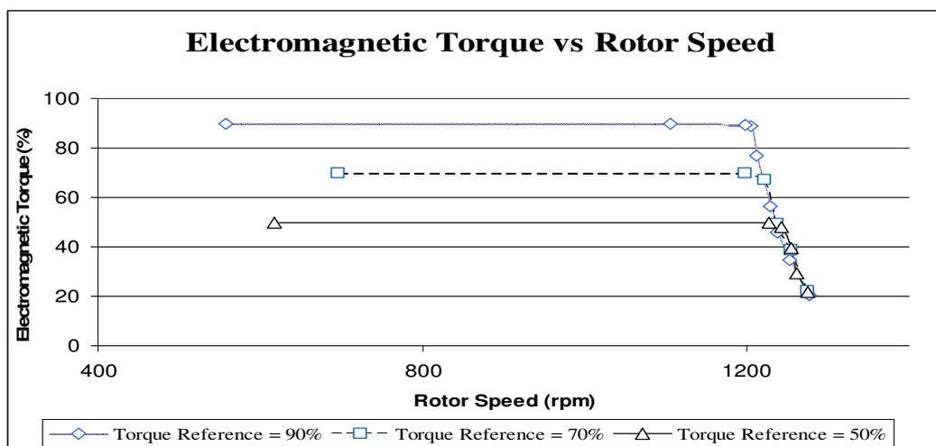
Figure 9: Rotor Speed vs. Electromagnetic Torque (Torque Control)
