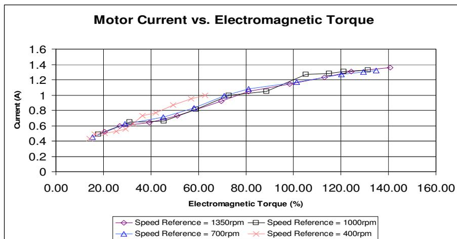
Figure 6: Motor Current vs. Electromagnetic Torque (Speed Control)
