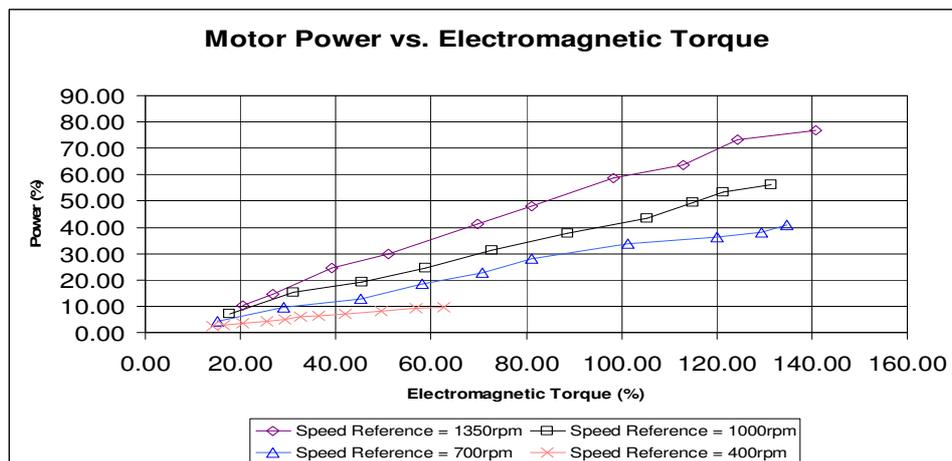
Figure 8: Motor Power vs. Electromagnetic Torque (Speed Control)
