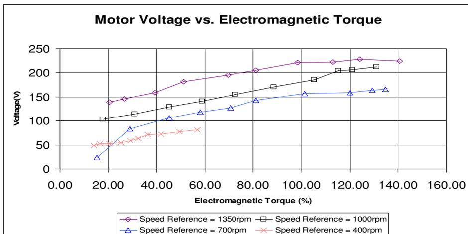
Figure 7: Motor Voltage vs. Electromagnetic Torque (Speed Control)
