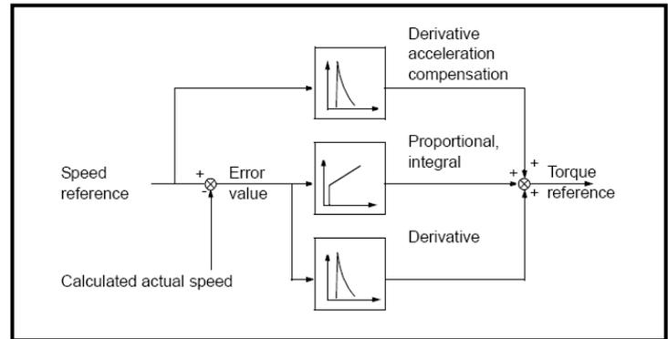
**Figure 4: Block Diagram of the Speed Controller**
