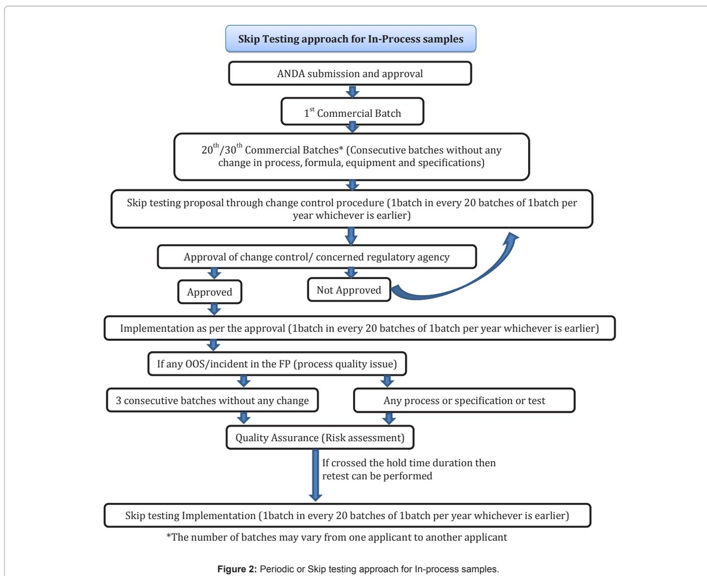
Figure 2: Periodic or Skip testing approach for In-process samples.
