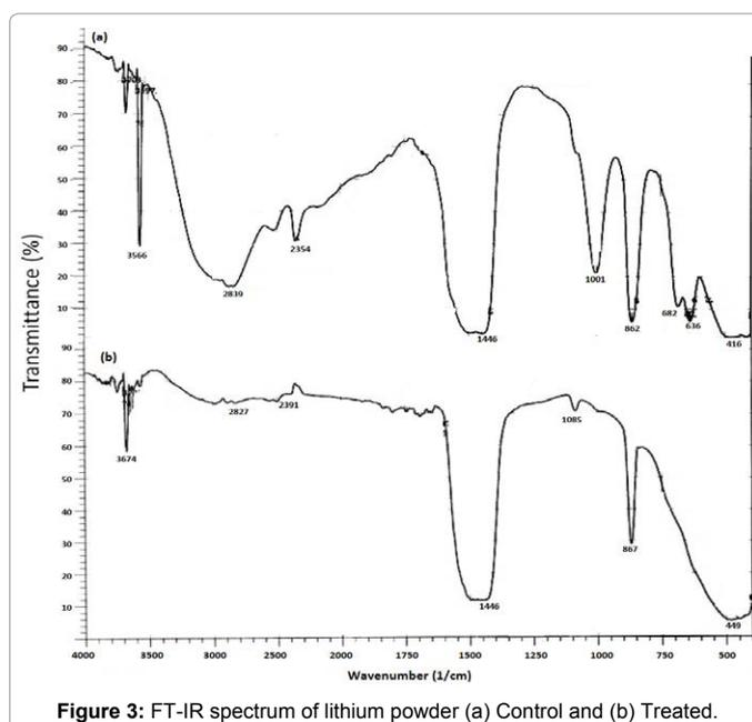
**Figure 3:** FT-IR spectrum of lithium powder (a) Control and (b) Treated.
