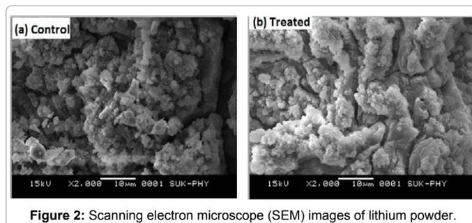
**Figure 2:** Scanning electron microscope (SEM) images of lithium powder.
