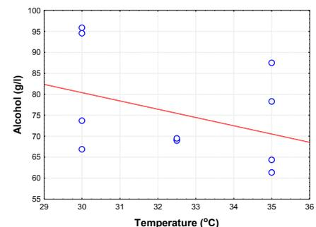
Figure 10: Relationship between alcohol generation and temperature.
