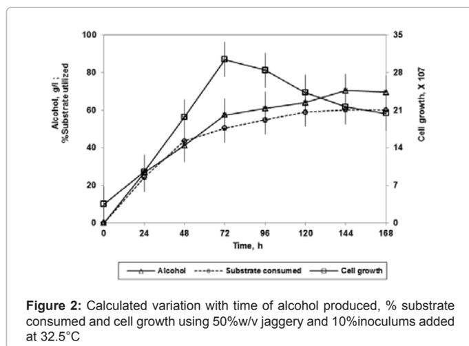
Figure 2: Calculated variation with time of alcohol produced, % substrate consumed and cell growth using 50%w/v jaggery and 10% inoculums added at 32.5°C
