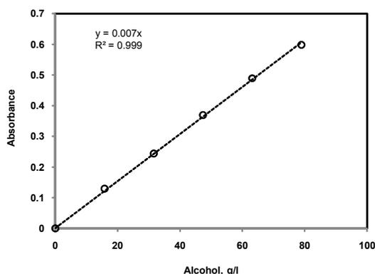
**Figure 1:** Standard calibration graph of alcohol by dichromate oxidation method.
