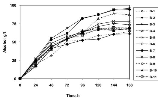
Figure 5: Alcohol generation kinetic in various batches during optimization process.
