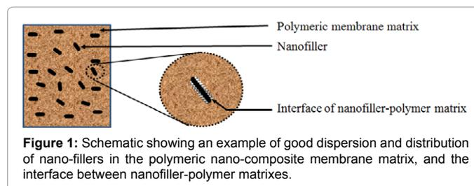
**Figure 1:** Schematic showing an example of good dispersion and distribution of nano-fillers in the polymeric nano-composite membrane matrix, and the interface between nanofiller-polymer matrices.
