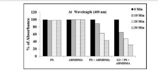
**Figure 5:** Combined results for all the three systems, showing decrease of OD at 400 nm (absorption maxima of ABMDMA) as a function of laser irradiation time.
