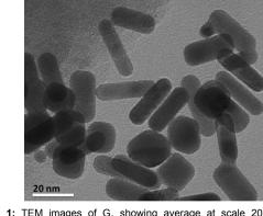
Figure 1: TEM images of  $\rm G_{2}$  showing average at scale 20 nm gold nanostructures.
