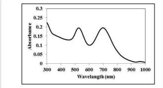
Figure 3: The Absorbance spectra of gold nanostructures.
