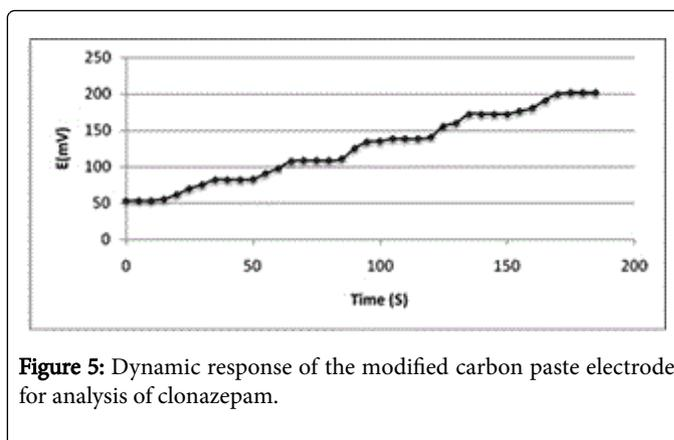
**Figure 5:** Dynamic response of the modified carbon paste electrode for analysis of clonazepam.
