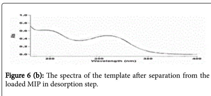
Figure 6 (b): The spectra of the template after separation from the loaded MIP in desorption step.
