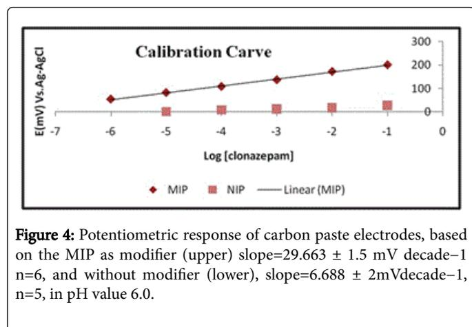
**Figure 4:** Potentiometric response of carbon paste electrodes, based on the MIP as modifier (upper) slope= $29.663 \pm 1.5$  mV decade<sup>-1</sup> n=6, and without modifier (lower), slope= $6.688 \pm 2$  mV decade<sup>-1</sup>, n=5, in pH value 6.0.
