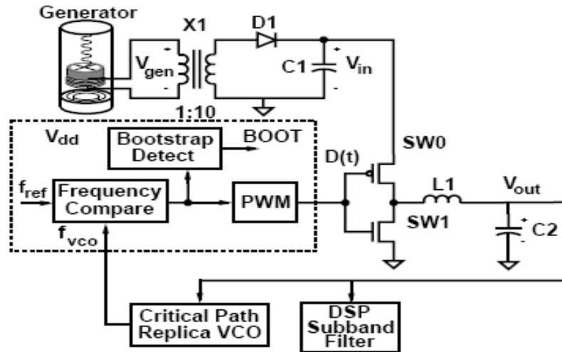
Figure 5(a): Vibration based self powered system
