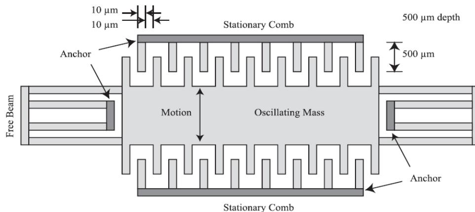
Figure 5(b): A plan view of MEMS generator
