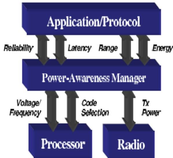
Fig8: Middleware convert communication performance requirement into optimal h/w settings
