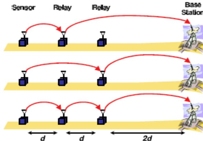
Figure 7(b): Three multihop policies when two nodes are b/w TX & RX
