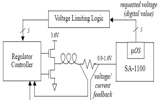
Figure 2: Regulation scheme for DVS
