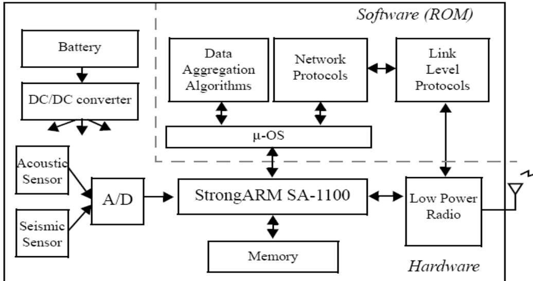
Figure 1: A sensor node hardware &amp; software framework
