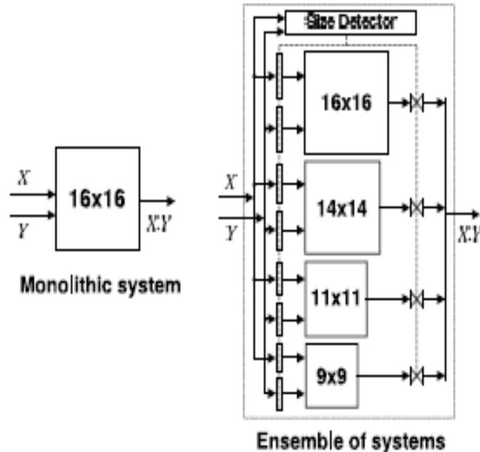
Figure 6: Comparison of Monolithic System and Ensemble of Systems
