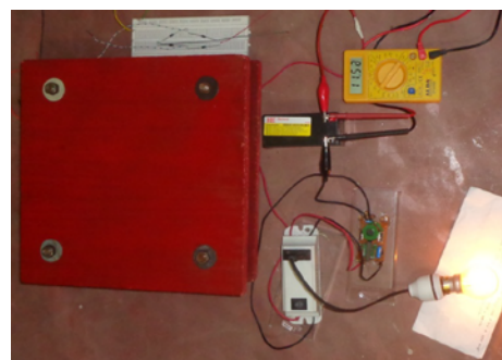
Figure 7: Connected a AC 5W bulb with inverter.
