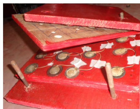
Figure 3: Design our project piezoelectricsensor.
