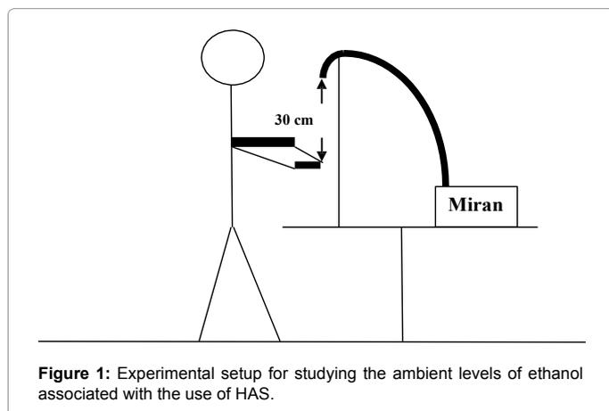
**Figure 1:** Experimental setup for studying the ambient levels of ethanol associated with the use of HAS.
