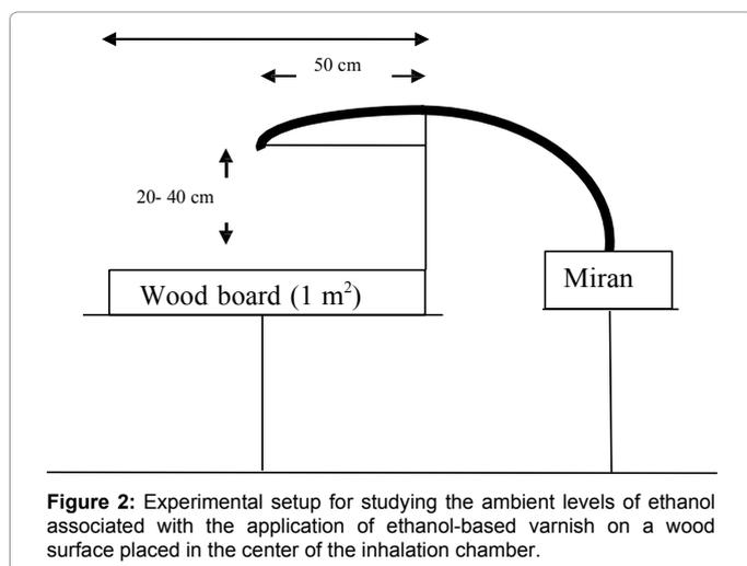
**Figure 2:** Experimental setup for studying the ambient levels of ethanol associated with the application of ethanol-based varnish on a wood surface placed in the center of the inhalation chamber.
