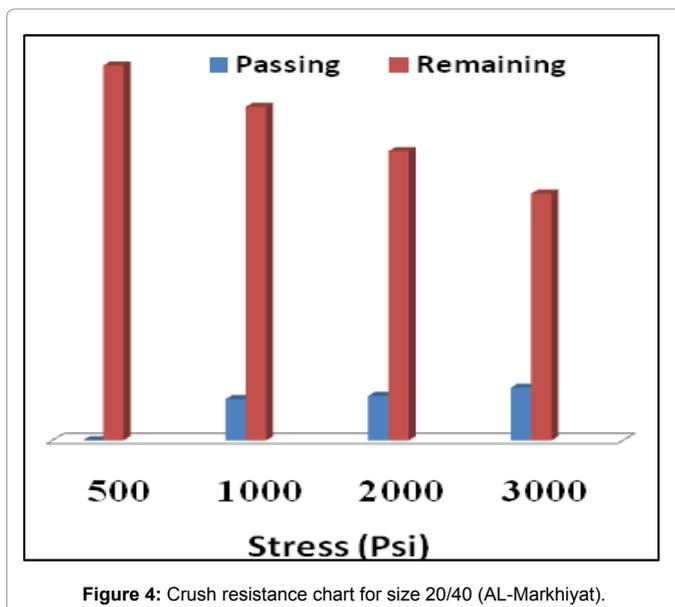
Figure 4: Crush resistance chart for size 20/40 (AL-Markhiyat).
