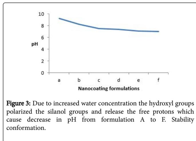
Figure 3: Due to increased water concentration the hydroxyl groups polarized the silanol groups and release the free protons which cause decrease in pH from formulation A to F. Stability conformation.
