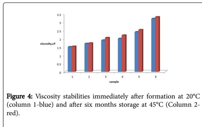
Figure 4: Viscosity stabilities immediately after formation at 20°C (column 1-blue) and after six months storage at 45°C (Column 2-red).
