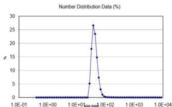
Figure 6B: Size measurement by Dls. Peak shows 11 nm size with 27% intensity. Precursor effect on particle size
