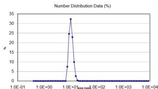
Figure 6A: Particle size was determined by light scattering method. Peak shows 1.2 nm particle size with 32.5% intensity.
