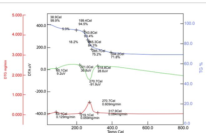
Figure 5: Thermogravimetric analysis of aluminum hydroxide, prepared by acid method of Tiger energy drink can. DTG=Differential Thermo Gravimetry, DTA=Differential Thermal Analysis, TG=Thermo Gravimetry.
