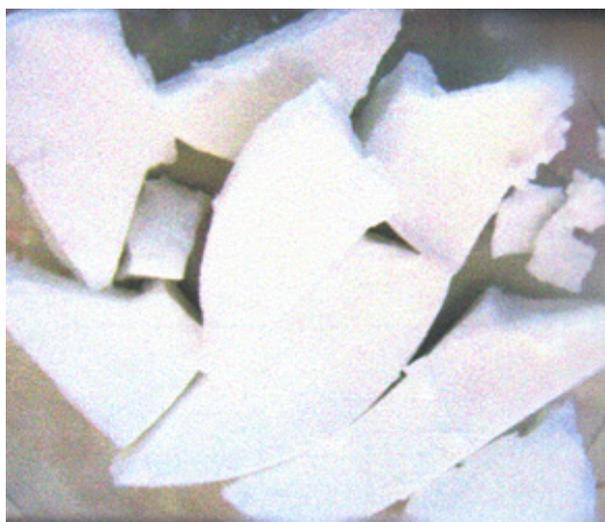
Figure 3: Aluminum hydroxide prepared in the laboratory.
