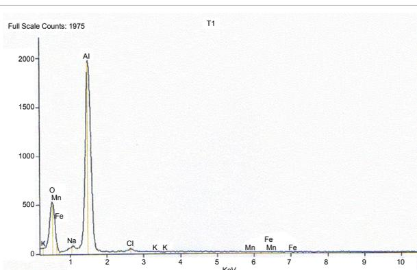
Figure 12: Spectrum of prepared aluminum oxide (acid method) by EDX.
