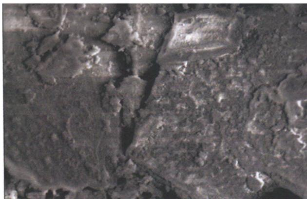
Figure 11: 1000 times magnification of aluminum oxide (alkali method of Tiger energy drink can).
