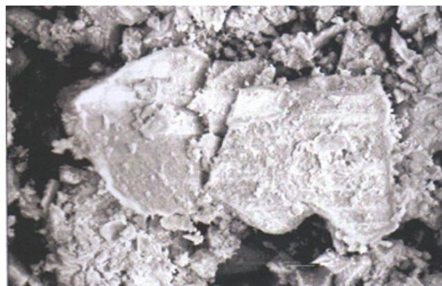
Figure 9: 500 times magnification of aluminum oxide (alkali method of Tiger energy drink can).
