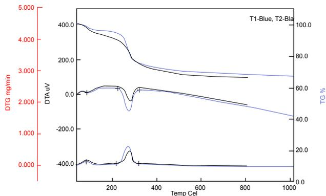
Figure 7: Comparative study of thermogravimetric analysis of two methods (acid and alkali).
