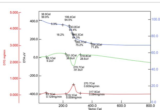
Figure 5: Thermogravimetric analysis of aluminum hydroxide, prepared by acid method of Tiger energy drink can. DTG=Differential Thermo Gravimetry, DTA=Differential Thermal Analysis, TG=Thermo Gravimetry.
