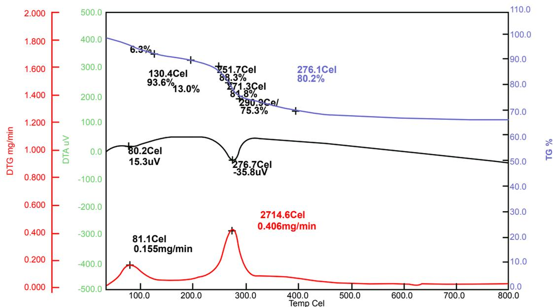
Figure 6: Thermogravimetric analysis of aluminum hydroxide, prepared by alkali method of Tiger energy drink can.
