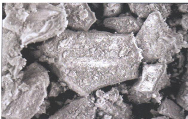
Figure 8: 500 times magnification of aluminum oxide (acid method of Tiger energy drink can).
