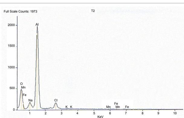
Figure 13: Spectrum of prepared aluminum oxide (alkali method) by EDX.
