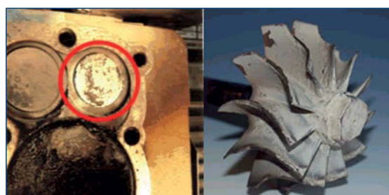
Figure 2: Incrustation on valves and turbines.
